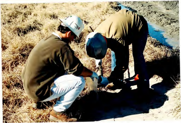
Figure 6. Bagging Samples. Pete Robinson, of Williams Environmental Services, removes CCBs from the auger for deposit into a sealable bag with the assistance of David Asti.
