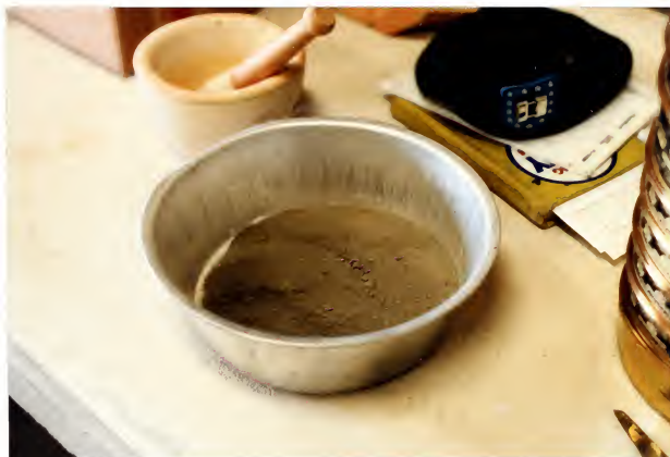
Figure 10. Size Distribution. All 15 samples from the moisture content tests were reused in the sieve analysis. After combining all the dried samples in this metal bowl a sample knife was used to break apart any particles stuck together from the drying process.
