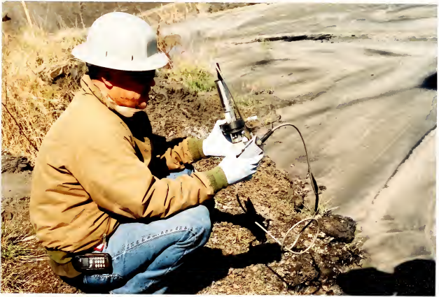
Figure 3. Field Testing of Permitted Discharge. A Hydrolab ® is utilized to test the permitted discharge close to the outlets from the discharge pipes. Note the grasses growing within the pond in the background of the photo.
