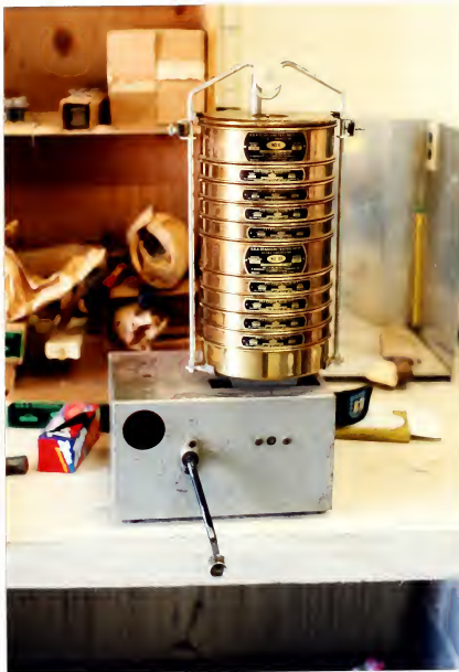
Figure 9. Sieve Analysis of CCBs. A manual agitator was used to shake the sieves during the analysis.
