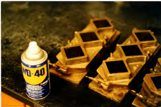
Figure 11. Cleaning the Mortar Cube Molds. The bronze molds for the mortar cubes required cleaning with a wire-brush. A light coat of oil was applied to act as a release agent to help remove the cubes from the mold after one day of curing.
