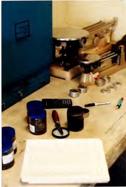
Figure 8. Soils Lab. Moisture content determination of the samples was done in the soils lab at the 926th Engineer Group, Montgomery, Alabama. Here a sample is being placed into tare #3 to be weighed, dried and reweighed. Electronic balances had to be used for certain measurements as the triple balance scale did not provide the precision some procedures required.
