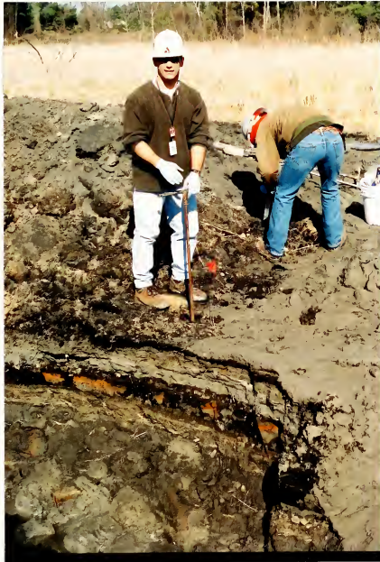
Figure 5. Hand Augering for CCBs Samples. David Asti of Southern Company is shown here sampling next to a dewatering trench excavated as part of the CCB stacking program. The stratification is visible within the trench. The thick black layer is the storm runoff from the coal stockpiles. The orange is iron oxide within the CCBs.
