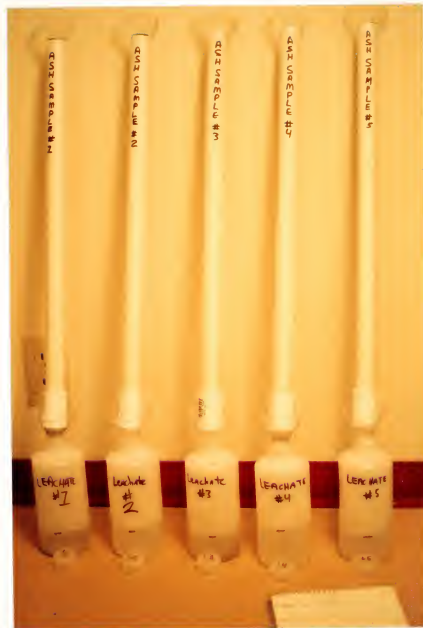
Figure 7. Open Column Percolation Apparatus. The amount of leachate within each of the collection bottles is after one week of percolation. The microscopic particle size (most < 45 \mu\text{m} in size) of the CCBs made an effective physical barrier to leaching even with only 3 inches of CCBs in the PVC pipe.
