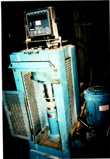
Figure 16. Hydraulic Cylinder Compression Machine. The compressive strengths of the 12 cubes were tested in this machine. The readout above the machine shows the total load applied to the face of the cube. This load would be divided by the area of the face of the cube to which the load was applied. The area of the face was calculated using measurements from a micrometer. This particular cube broke at 28 days with a strength of 2,600 pounds per square inch (psi).
