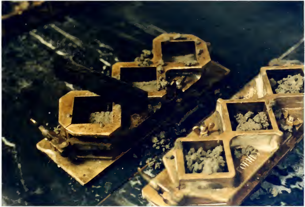
Figure 13. Tamping the Mortar. Air bubbles within the cubes had to be eliminated or else they would weaken the cubes. A rubber tamper was utilized in accordance with the tamping procedure outlined in ASTM C 109-99.
