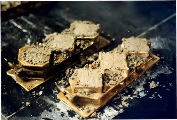
Figure 14. Tamping Completed. After each of the three layers of mortar is placed within the mold they are tamped. Here are the molds after the third layer is tamped. Notice there is still some excess above the top of the mold. That excess was removed by screeding, or scraped off, across the top of the mold with the tamping tool.
