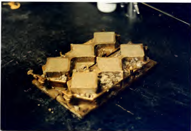
Figure 15. Finished Cubes. After screeding the tops of the cubes with the tamping device these cubes were then cured at room temperature for 24 hours before being moved to a water bath at Geosciences Lab in Columbus, Georgia where they would undergo compressive testing in 7, 14, and 28 days.
